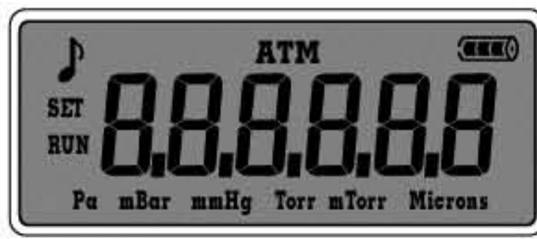
真空度单位: Pa, mBar, mmHg, Torr, mTorr, Microns VACCUUM UNITS: Pa, mBar, mmHg, Torr, mTorr, Microns
